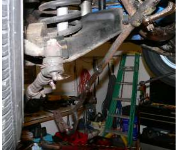
UNBOLT IDLER ARM & INNER TIE ROD ENDS
